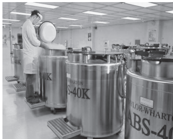
Fig. 2 Liquid nitrogen (LN 2 ) storage in BCRC/FIRDI. BCRC offers secure and reliable safe deposit for valuable microorganisms, cell lines and related materials. In response to the increase in natural disasters due to climate change, BCRC has constructed a remote site for maintaining the back-up collections.
